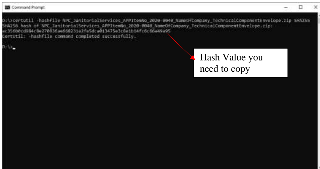
Figure 4. Hashfile command in Command Prompt
